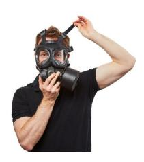
3. Once the harness has been secured. Cover the exhalation opening of the respirator with your hand. Exhale gently to create overpressure. There must be no leakage between the face and the face seal.
