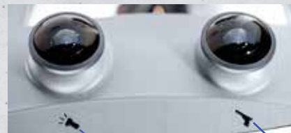
Simulator for Law Enforcement has two cameras: flash light and firearm
